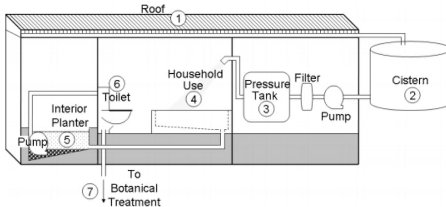
**Figure 5. Earthship catchwater and greywater system.**
