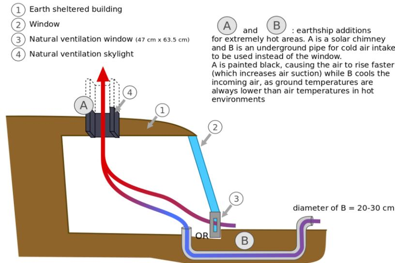
**Figure 2. The Stack Effect (Thermal Draught).**
